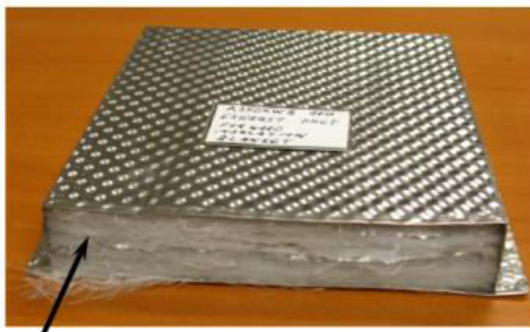
Figure 2 – Typical thermal blanket for exhaust mufflers
