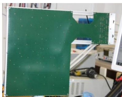
Figure 2: Example of microphone array containing 64 sensors.
